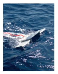
Figure 3.4 Manta net being used to collect microplastics from surface waters in the Pacific, operated from S/V Kaisei, 2009. Image courtesy of Doug Woodring, Project Kaisei; http://projectkaisei. wordpress.com/the-science-team/.
