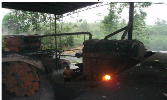
This antiquated Chinese tyre pyrolysis plant is hardly the sort of facility that receives government approval
