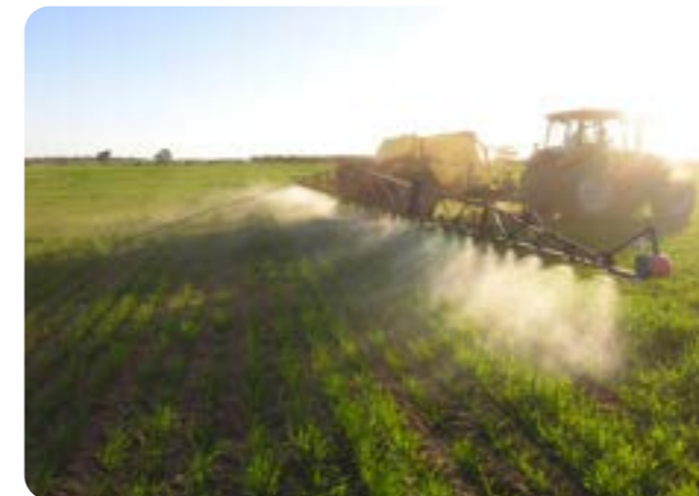
Pesticide boom sprayer. Image by the Department of Agriculture and Food WA.
