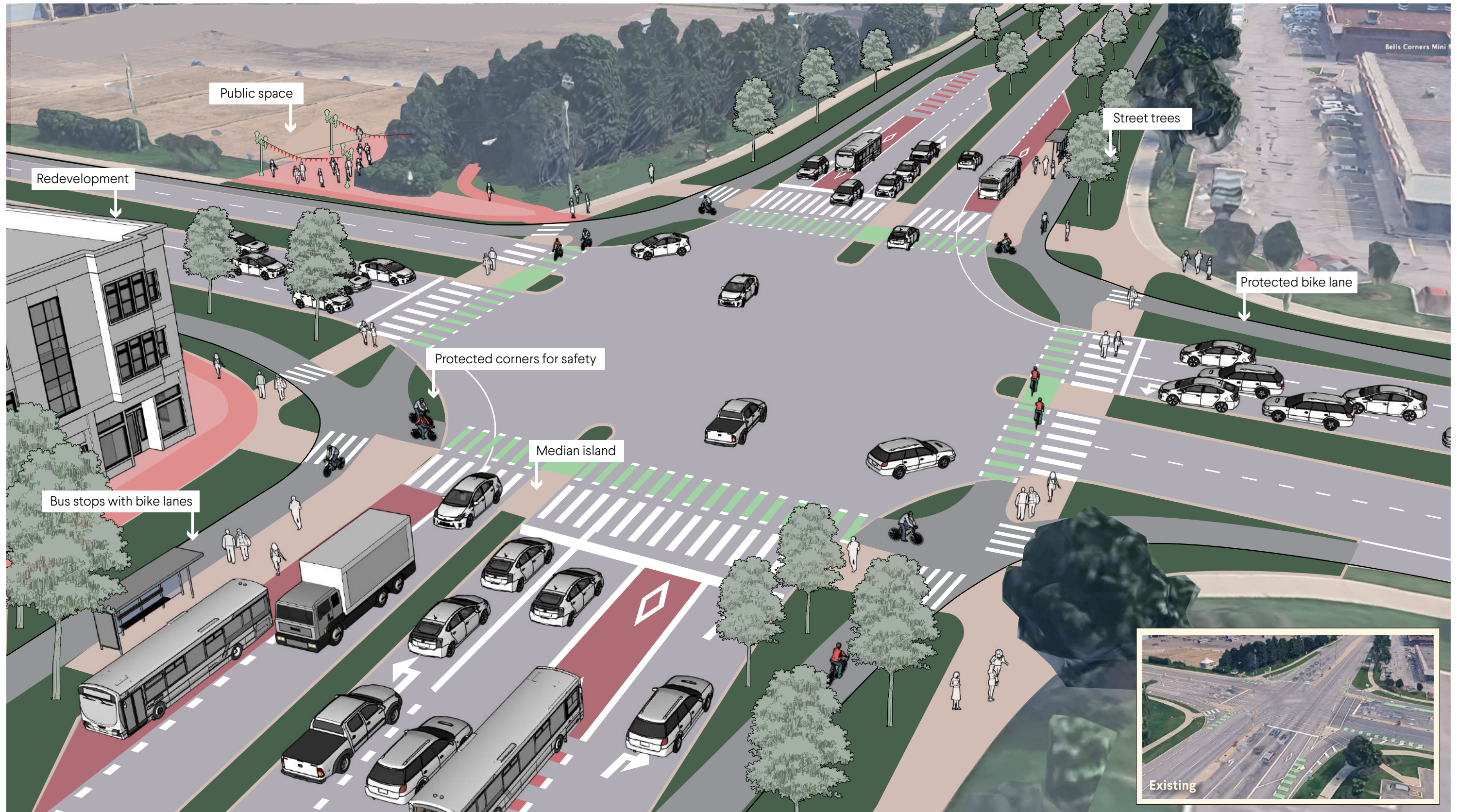
Figure 7. An illustration of how some of the design principles could lead to a larger transformation of the street through a corridor study, with safer places to walk and cycle, priority for transit, major investments in streetscaping, and the construction of new buildings.
