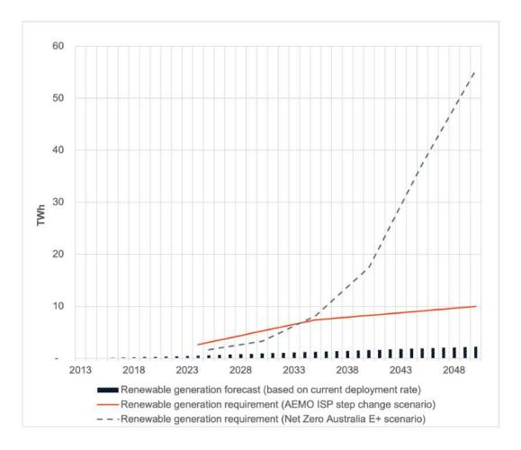
The build rate modelled has been calculated based on Clean Energy Council data using an average of the large-scale renewable generation capacity reaching commissioning over the last five years and APVI data on annual rooftop PV deployment [5] [10]
