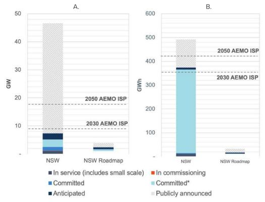
The potential storage capacity of the NSW Roadmap is shown with the same project status classifications to understand its role in the overall pipeline.
