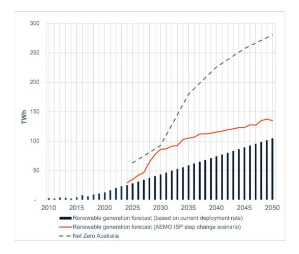
The build rate modelled has been calculated based on Clean Energy Council data using an average of the large-scale renewable generation capacity reaching commissioning over the last five years [5] and APVI data on annual rooftop PV deployment [10].
