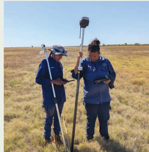
Romaniah Hunter and Gaydar Lawford conducting ground truthing surveys using point intercept method pairs with highly accurate GPS data collection.
