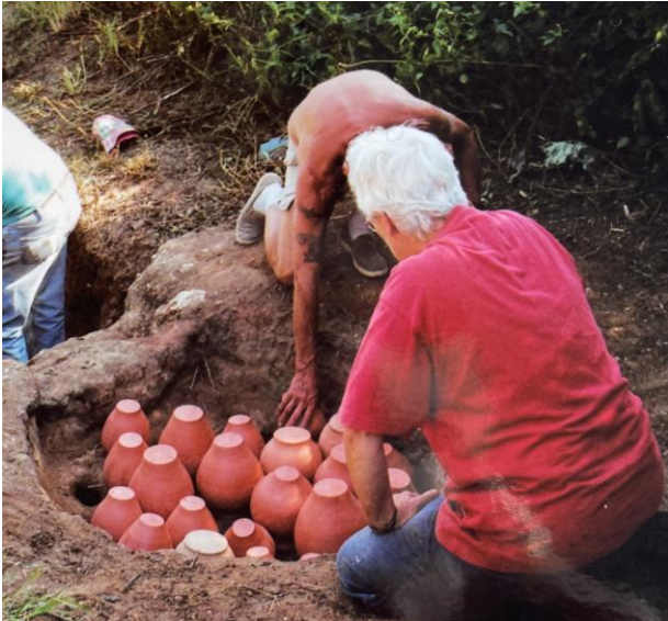
Stacking the pots (already biscuit fired) in the kiln on top of the perforated clay floor, before the fire is lit.
