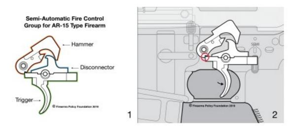
The hammer is spring-loaded, storing energy as it is moved rearward into the "cocked" position. The trigger keeps the hammer in the "cocked" position by way of its "sear," a geometric plane that locks the
