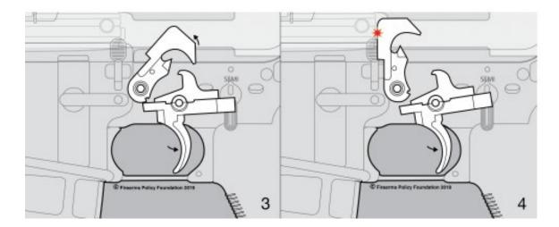
In a semiautomatic firearm, the bolt re-cocks the hammer. By the time the bolt reciprocates, the operator may still have the trigger depressed. This is where the "disconnector" comes into play. When the trigger is depressed, the disconnector moves into its active state. Image 5. When the weapon fires, the bolt travels rearward, pushing the hammer to the rear. The disconnector captures the hammer near its rearmost position. Images 6.
