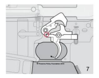
Were it not for the disconnector, upon firing, the bolt would push the hammer rearward, but as the bolt returned forward under spring pressure, the hammer would "follow" the bolt as it returns to battery, failing to re-cock the hammer or to strike the firing pin with sufficient force to discharge a subsequent round. Absent extraordinary circumstances, this creates a need to manually re-cock the hammer.
