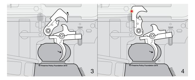
While the empty casing is being ejected from the firearm, the bolt carrier slides rearwards and the hammer is pushed back towards the disconnector. The disconnector grabs and holds the hammer, preventing it from firing another round
