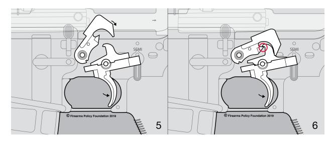
A second function of the trigger occurs when the trigger is released causing the disconnector to let go of the hammer, which then again rests on the "reset" edge of the trigger, awaiting the next function of the trigger to initiate the next firing sequence. Image 7.
