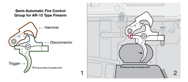
When the firearm is set to fire, the hammer rests on the internal edge of the trigger. Image 2. Pulling the trigger – a single function – releases the hammer, which strikes the firing pin and results in a single round being discharged. Images 3-4.
