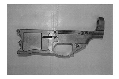
116. The January 2017 ATF letter determined that a Glock-type frame identified as a "PF940C Blank" was "not sufficiently complete to be classified as the frame or receiver of a firearm" because six specified machining operations or design features were "not yet present or completed." The letter included the below picture illustrating ATF's conclusion that the weapon presented in this picture was *not* a firearm:
