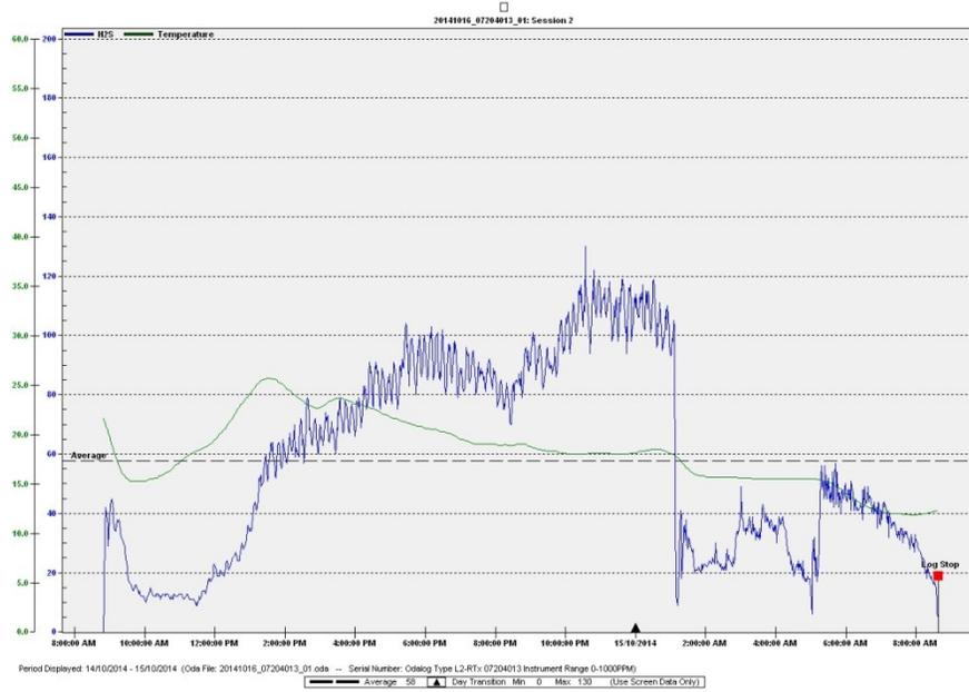
**Figure 1 – Data Logged Results of H<sub>2</sub>S Concentration with no Odour Control**
