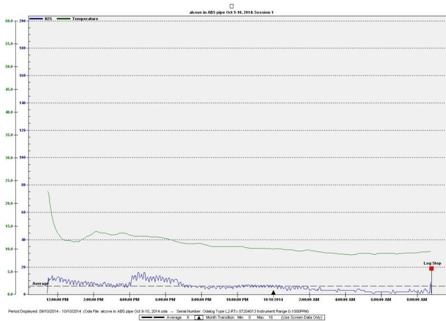
**Figure 2 - Data Logged Results of H<sub>2</sub>S Concentration with two Odorox MVP 14 Hydroxyl Generating Odour Control units**
