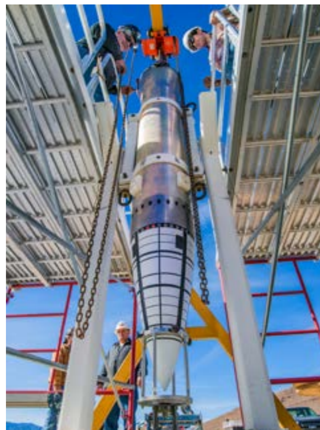
The nose assembly of a mock B61-12, mounted on an aluminum tube to replicate the body of the bomb, sits in a stand awaiting movement to Sandia National Laboratories' Davis gun, which fired the test assembly into a pool in one of a series of impact tests. Photo: US Department of Energy.
