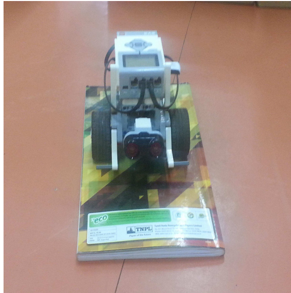
Figure 6: Lego Mindstorms kit assembled as a Cart.
