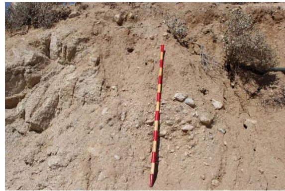
Figure 18 Location A; Roadcut exposure showing fine-grained debris flow incorporating lens of channel lag. Edge of channel defined by crystalline rock to left of staff. Staff marked in decimeters.
