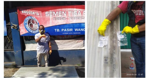
Sampling & Testing Potential ACM (Asbestos Containing Materials)
