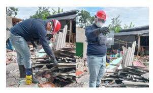
LION also conducted mapping and took samples of damaged asbestos-containing materials at various earthquake affected locations. The results have been taken for laboratory testing and will become important evidence for future research and policy advocacy related to controlling and eliminating the risk of asbestos exposure, especially in post-disaster areas.
