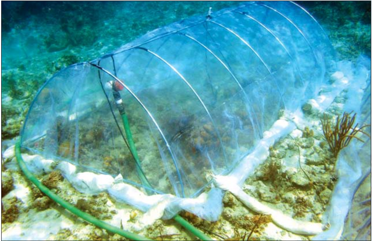
Underwater respirometry devices like the one shown are used for studying ecosystem function in the Tampa Bay Study. U.S. Geological Survey.
