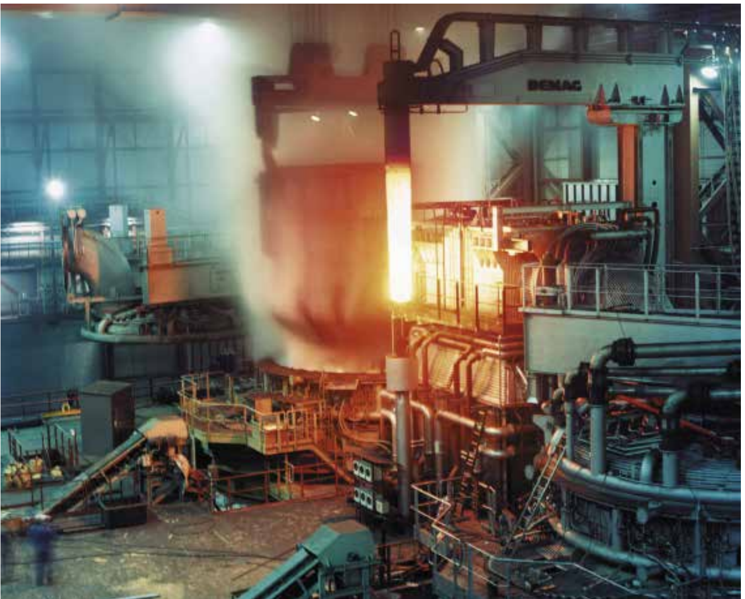
Electric Arc Furnace (Photo: ArcelorMittal)
