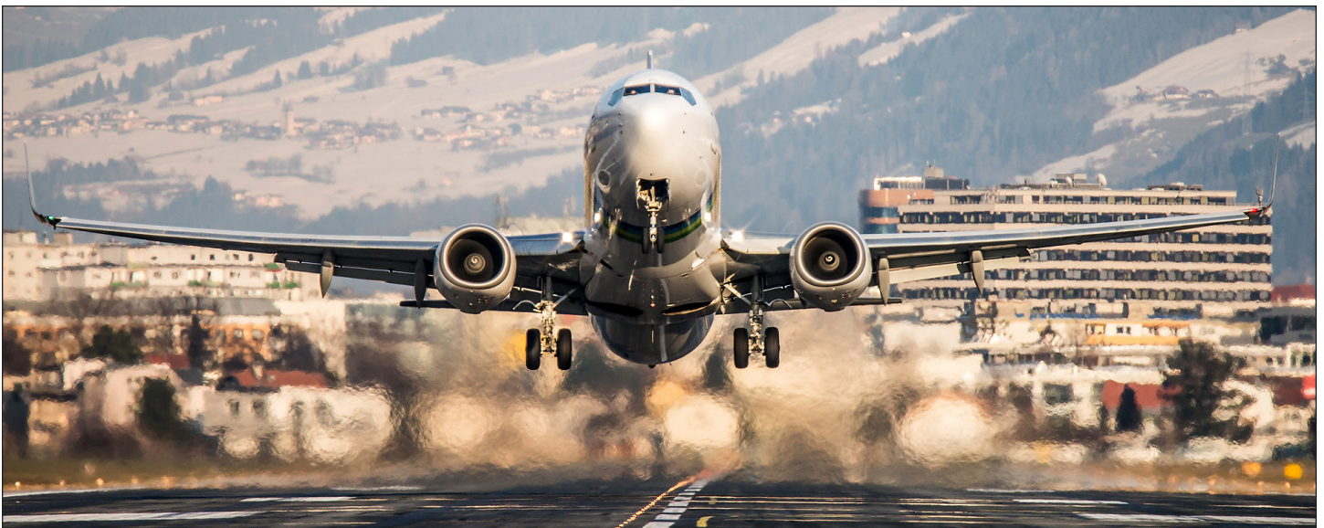
Middle image: Actual photo of wake turbulence (not normally visible unless atmospheric conditions are right as in this image).
