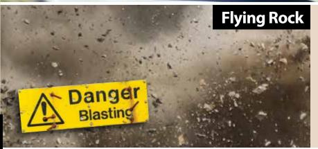
Flying rock is rock fragments propelled through the air beyond the normal blast zone by explosives detonated to fragment the rock.
