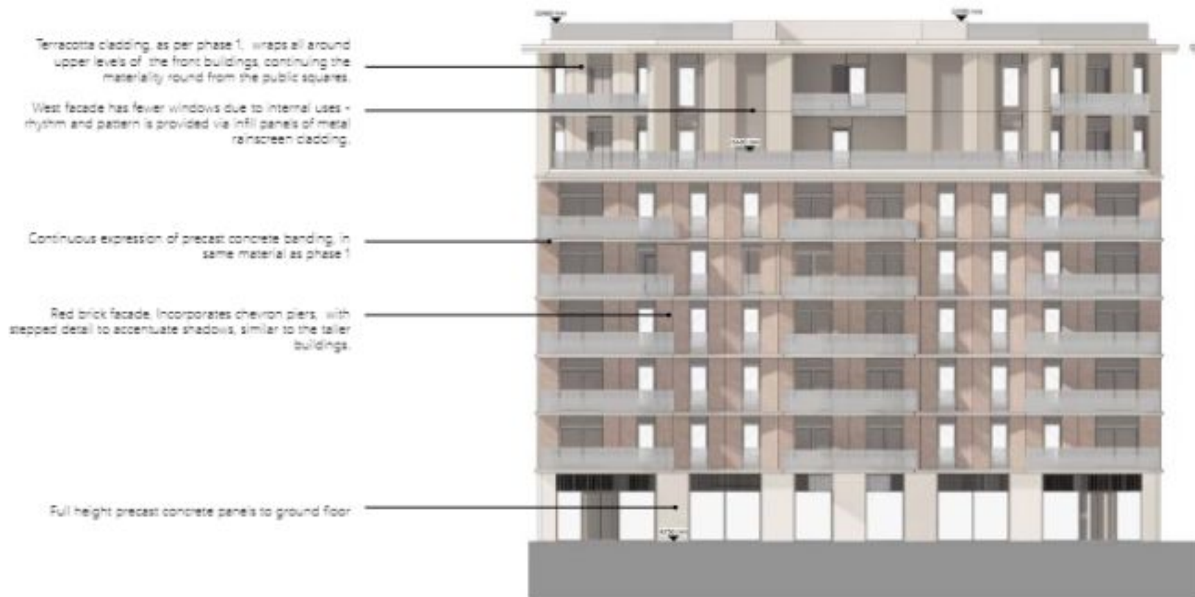
West: Ebury Bridge Road Street frontage:
